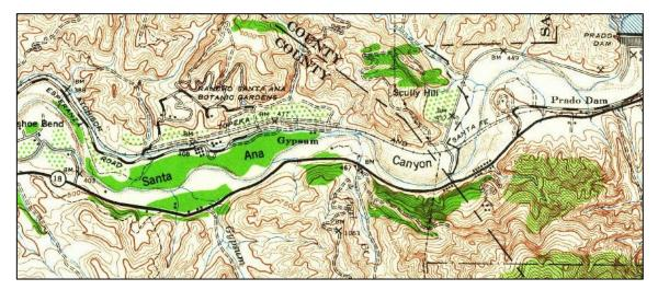
Figure 6-3 ATSF Rail Line through the Project area in the Santa Ana Canyon. Note the new, more direct route through the Project area built after the 1939 flood and to facilitate the construction of the Prado Dam (USGS 1942).
